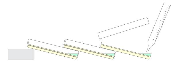
Figure 1: Tilting and stacking plates to assist with aspiration of concentration lysate.
